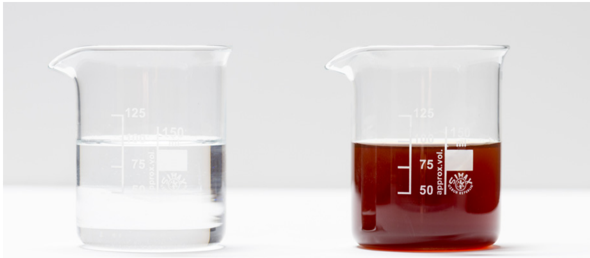
Figure 6. First flush drain water from GRODAN substrate (left) compared to coco (right).
