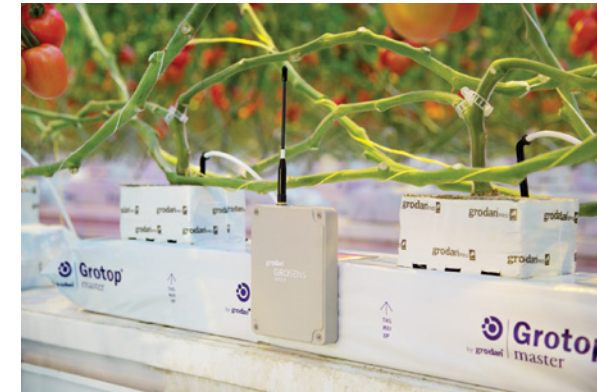
Picture 2. GroSens helps growers make informed root zone management decisions
